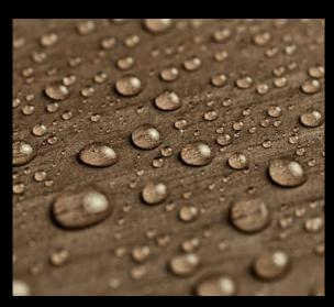
The closed surface created by Trespa's proprietary Electron Beam Curing (EBC) technology makes it hard for dirt to build up, locking it out and colours in.
